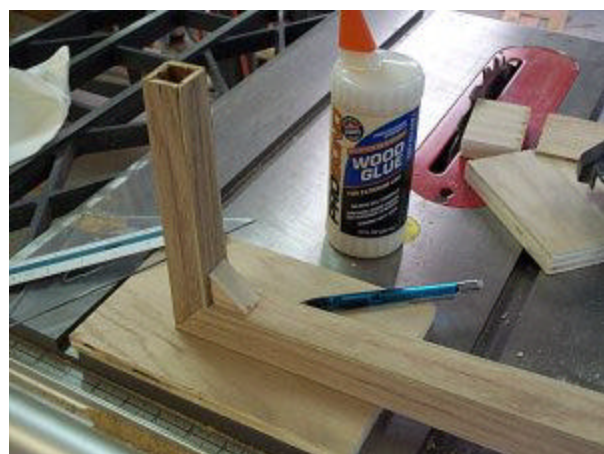
BDU Tube's Bocal subsection with wooden wedge
