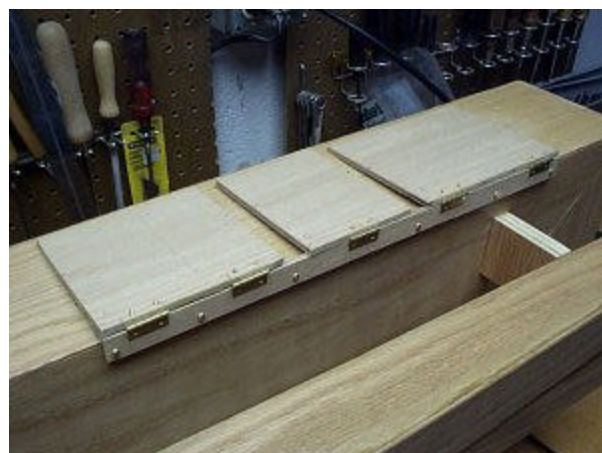
keys mounted to hinge rail for lower hole group
