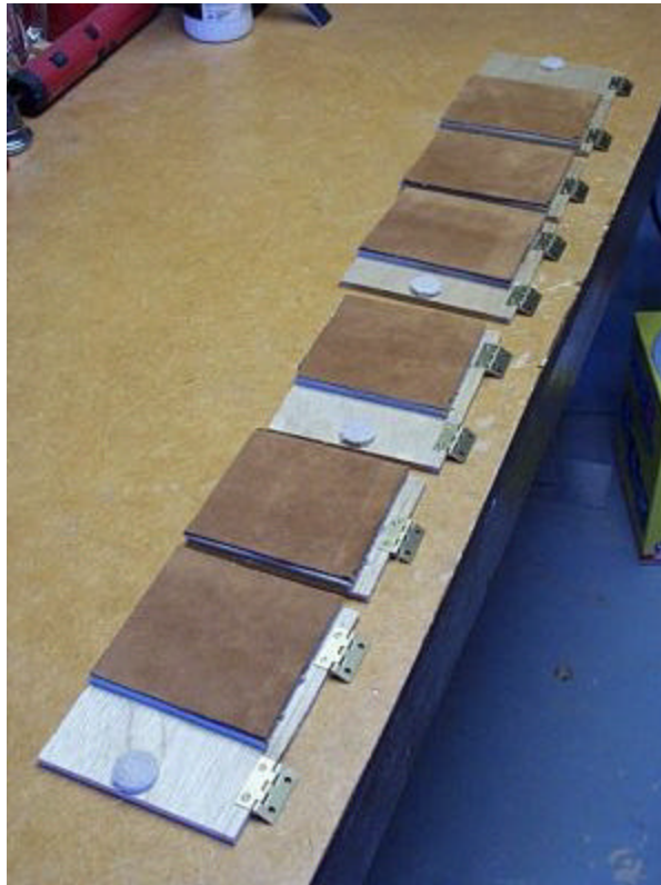
keys with bumpers & pads trimmed short of hinges
