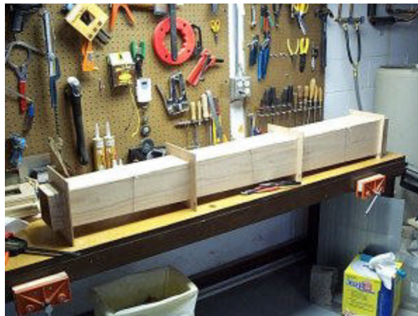
Bell Tube section glued with outer jigs visible
