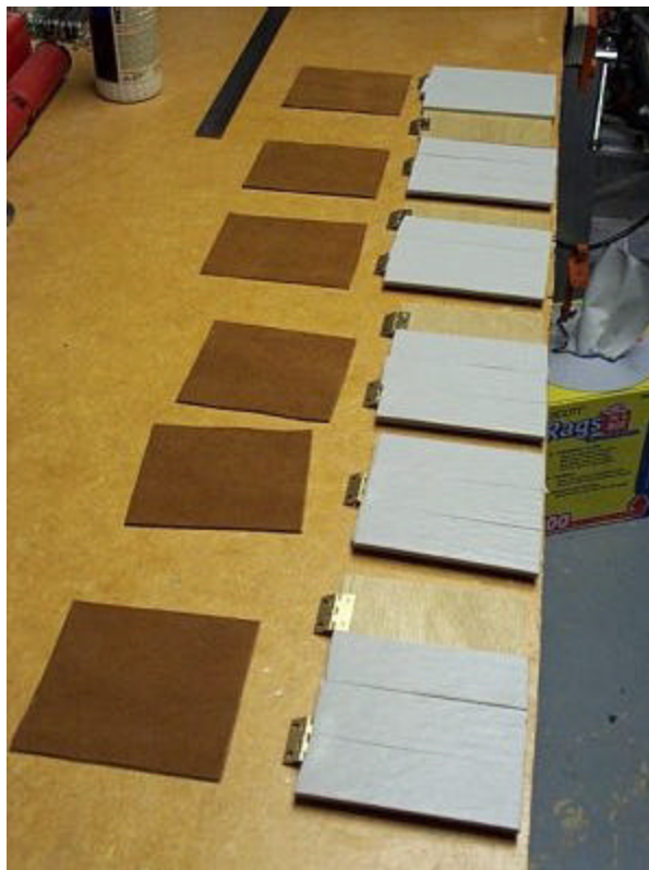
keys with foam attached and ready for leather
