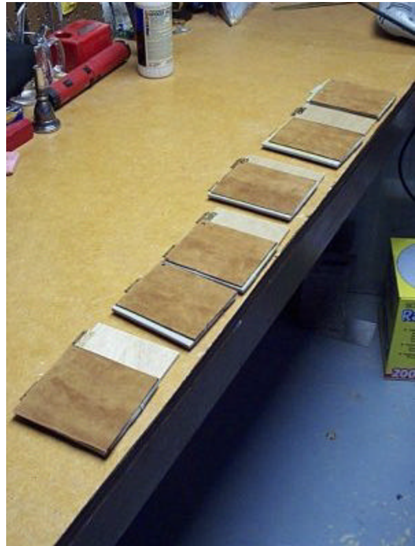
keys with leather glued to foam
