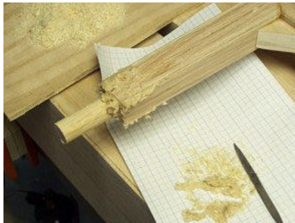
dowel epoxy-ed into Bocal's receiver
