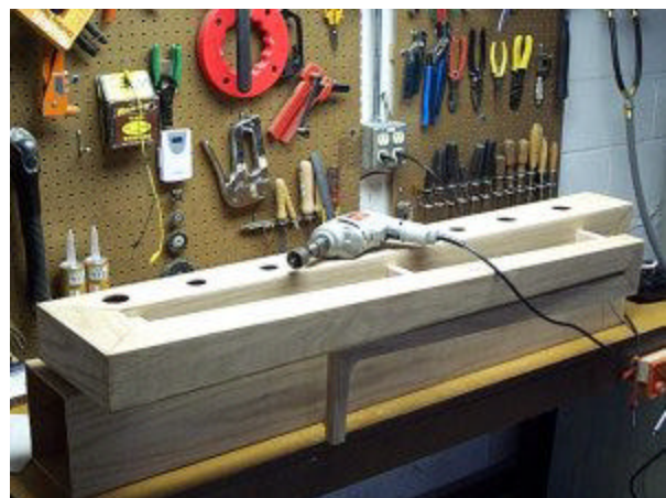
a drill operated hole saw and six completed holes
