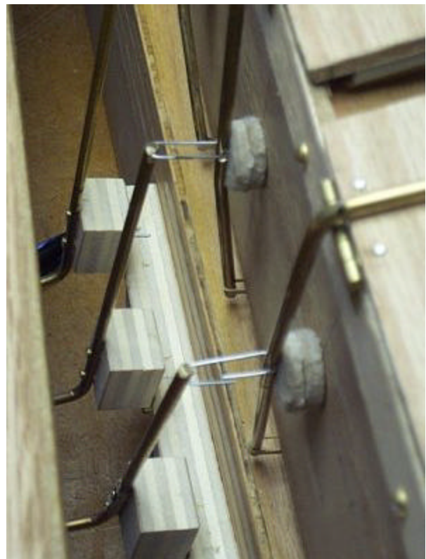
levers and linkages for lower hole group
