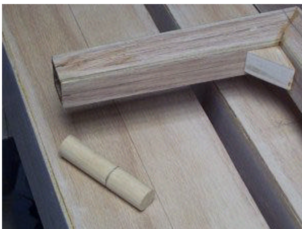
Bocal and receiver dowel with 1" mark
