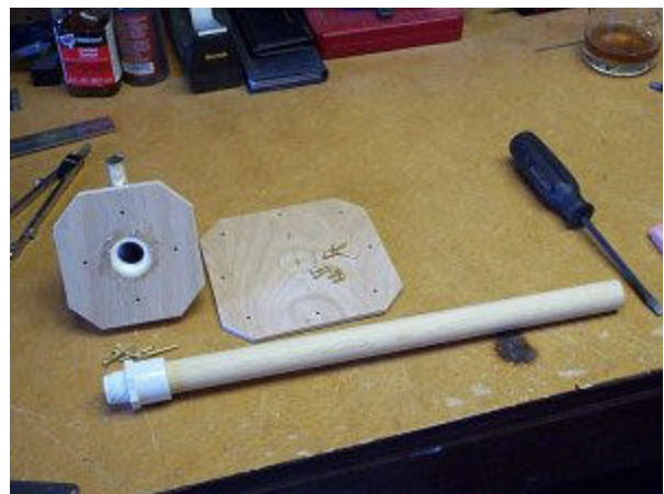
peg parts after gluing fittings to wooden parts
