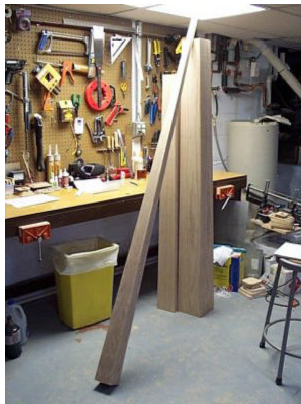
all three sections with outer jigs removed
