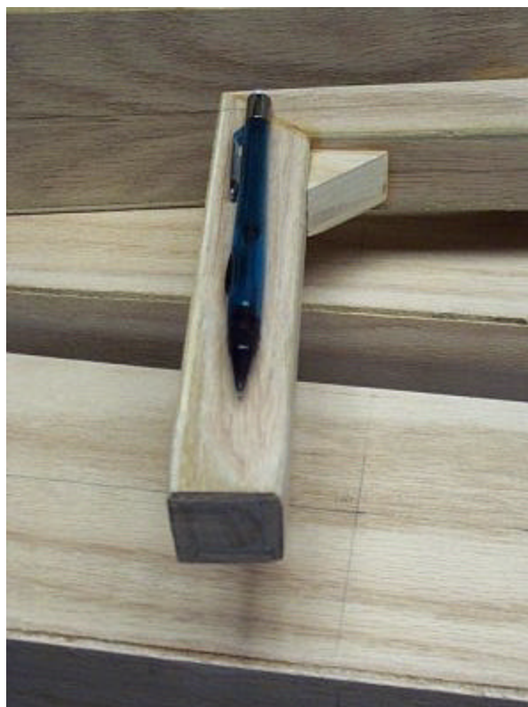
receiver with excess dowel cut off
