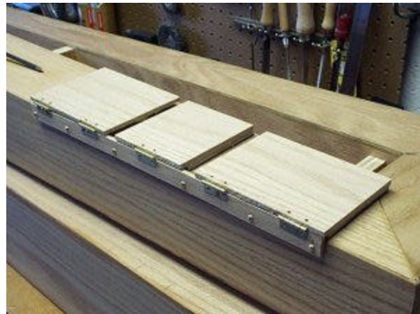
keys mounted to hinge rail for upper hole group
