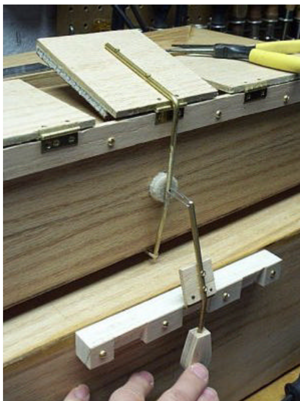
first key lever completed; the left photo shows the key open and the right shows it closed - the button lever is shown flipped upside down from the final design's orientation
