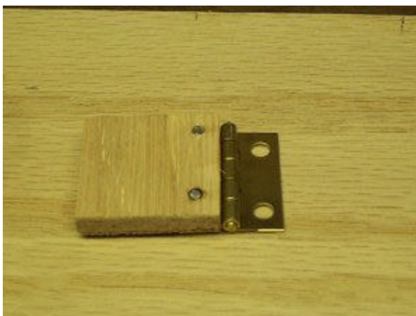
hinge tab (thin version for upper key group)
