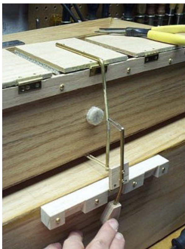
first key lever completed; the left photo shows the key open and the right shows it closed - the button lever is shown flipped upside down from the final design's orientation
