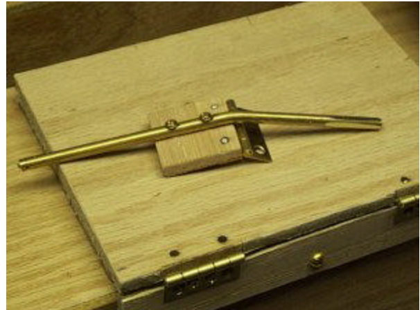
hinge tab (thin version) with second part of lever pair attached
