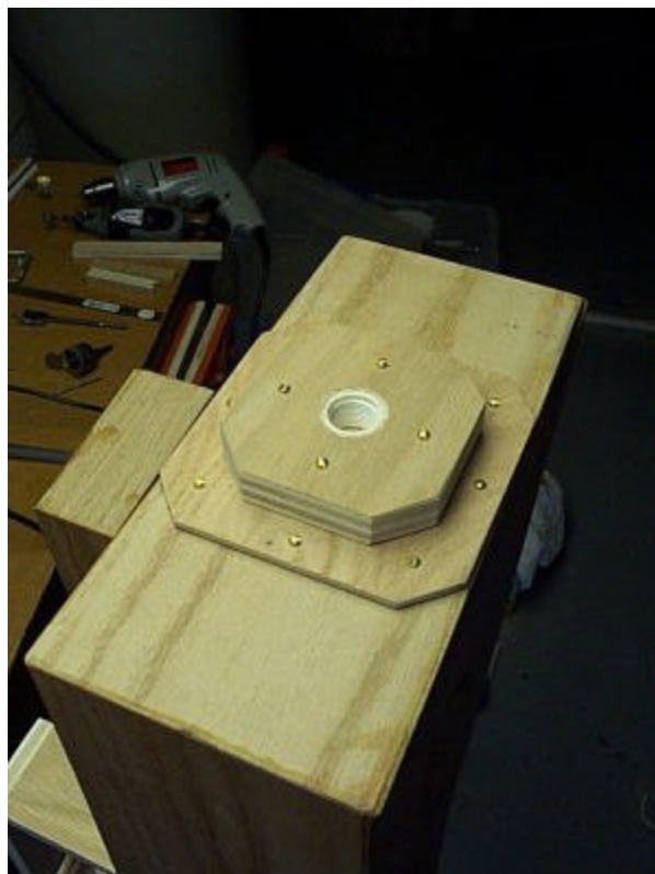
peg anchor screwed to bottom end of CBS
