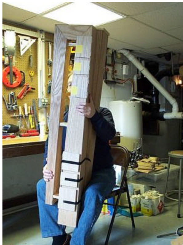
testing key pad seals, with keys taped closed
