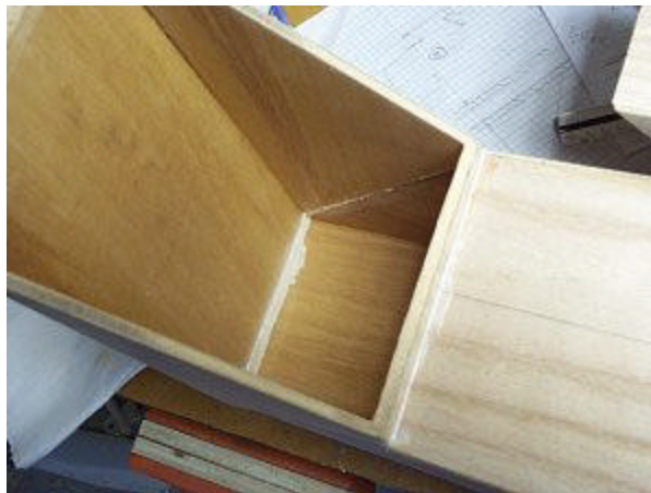
typical gluing of tube bend
