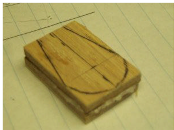
button laminated and marked for cutting
