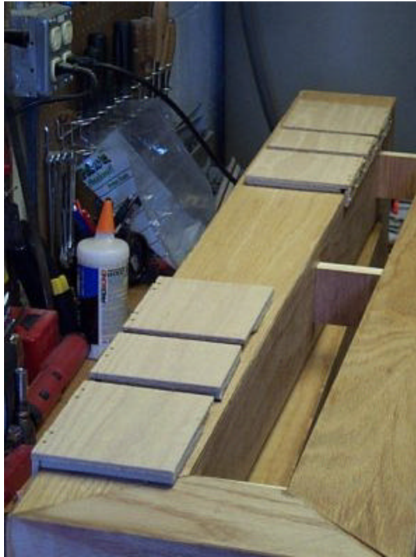
all six keys mounted; note how each group is mounted on the opposite side of the Key Tube
