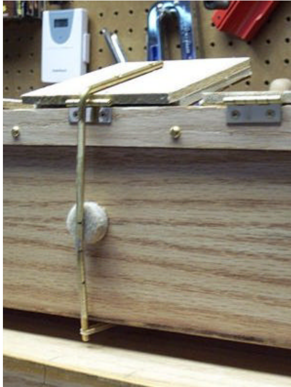
first half of lever pair, with felt bumper and rubber band spring
