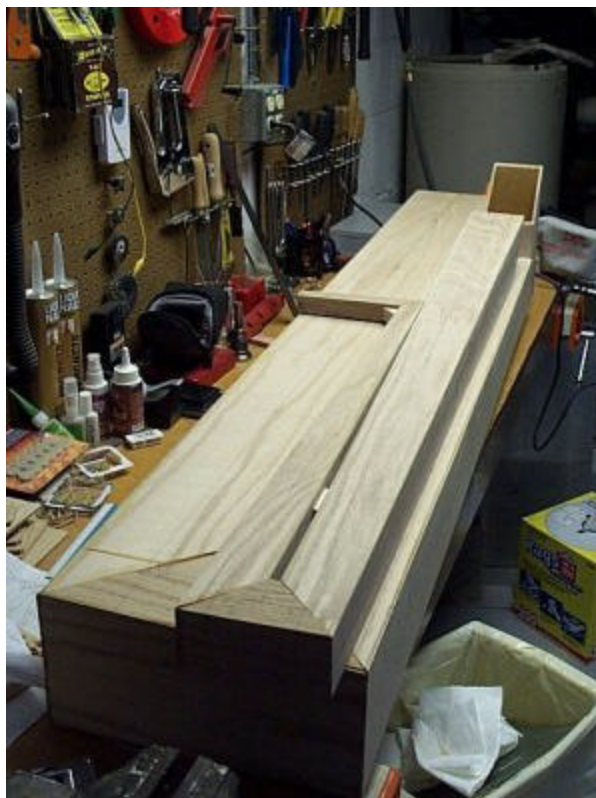
reshaped BDU Tube assembly ready for mating to reshaped Key / Bell Tube assembly
