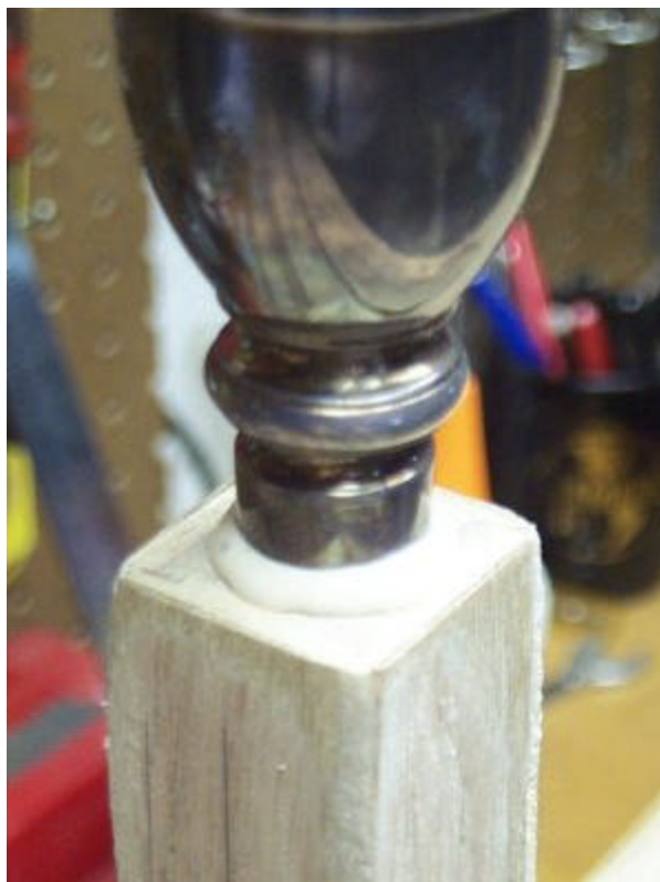
forming the caulk receiver fitting
