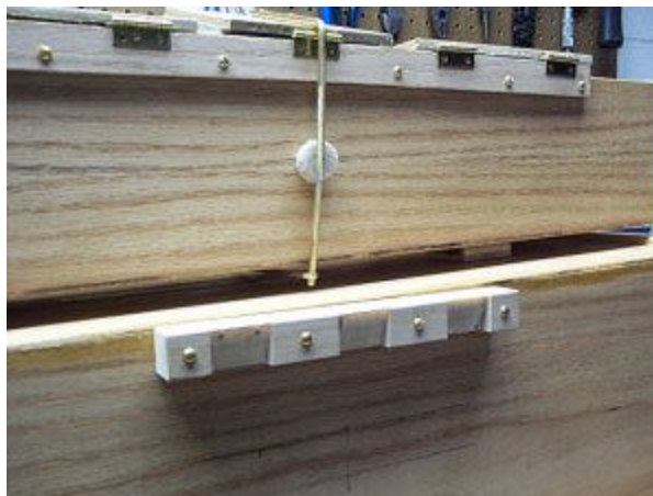
hinge block (beveled cuts are not required)
