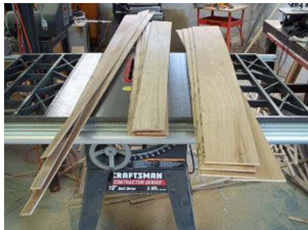
12 trapezoids after cutting from plywood sheets
