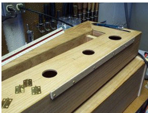
hinge rail mounted for upper hole group
