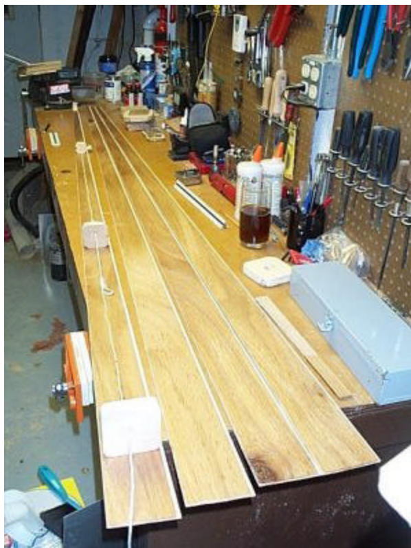
inner jigs in place on trapezoid, with cord
