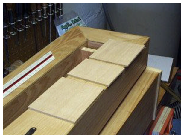
plywood keys test fit for upper hole group; they are still too wide
