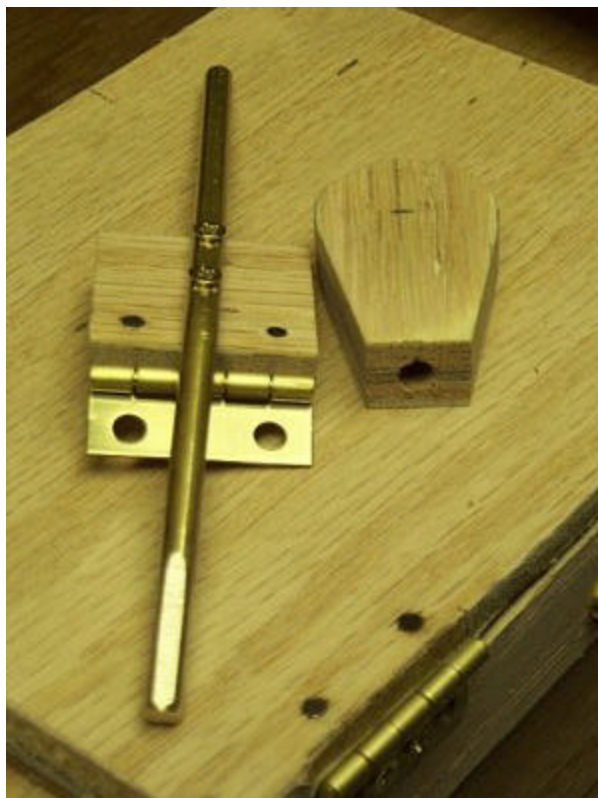
hinge tab with lever and button ready for mounting
