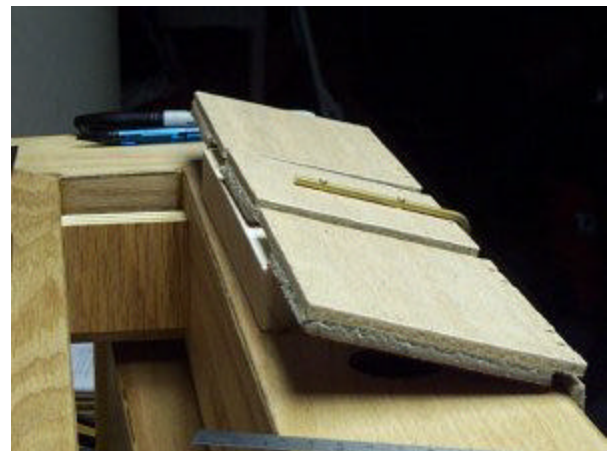
1" wood block holds keys open for fitting levers
