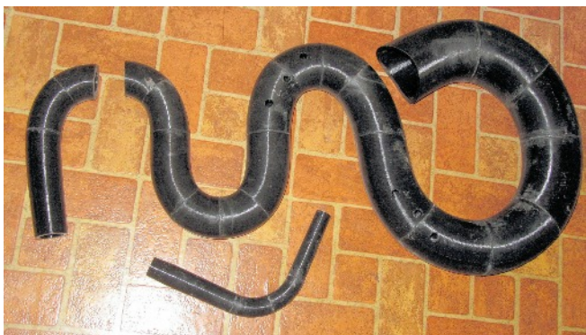
Dorsey/Witkowski 3D printed serpent, after Bate #504, as received with separated joint, and its detached bocal. Note discoloration at each joint due to use of CA glue accelerant
