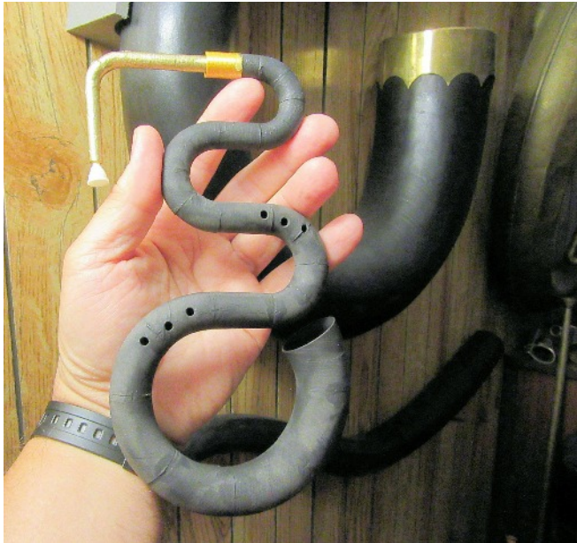
Completed 3D printed "Worm" with correct scale bocal and mouthpiece fitted, bocal and body painted, posed in front of part of a Monk Military Serpent
