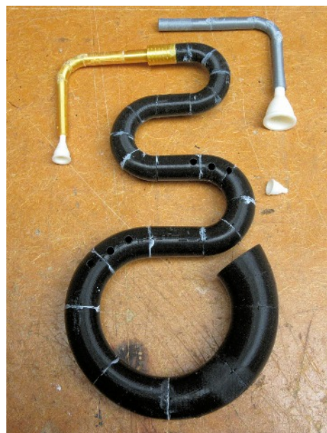
3D printed "Worm" assembled, plus special adapter bocal to fit 50% scale mouthpiece to make playing possible
