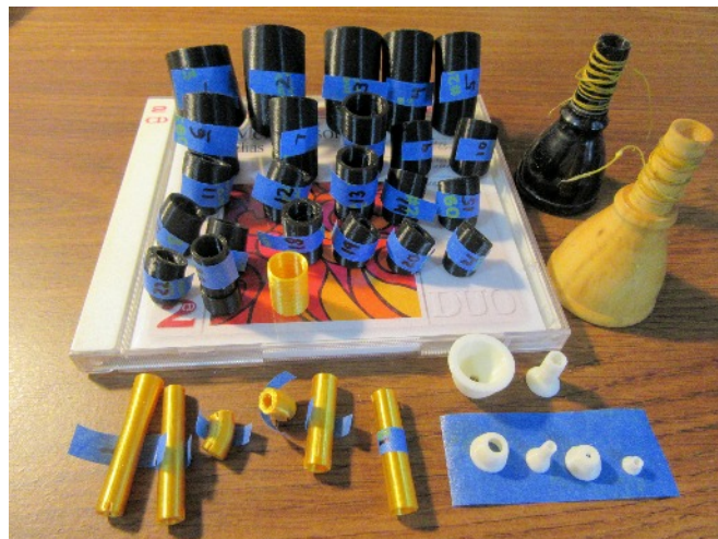
All of the 3D printed pieces of a 1/4 scale (25% full size) church serpent after Bate # 500 "Dittes", as required to make a "Worm". The pieces are posed on a typical audio CD 'jewel box' case for scale, and two 'real' serpent mouthpieces in horn and boxwood are adjacent. Two halves each of two different 25% scale serpent mouthpieces are on blue tape, while two halves of a 50% scale mouthpiece are adjacent
