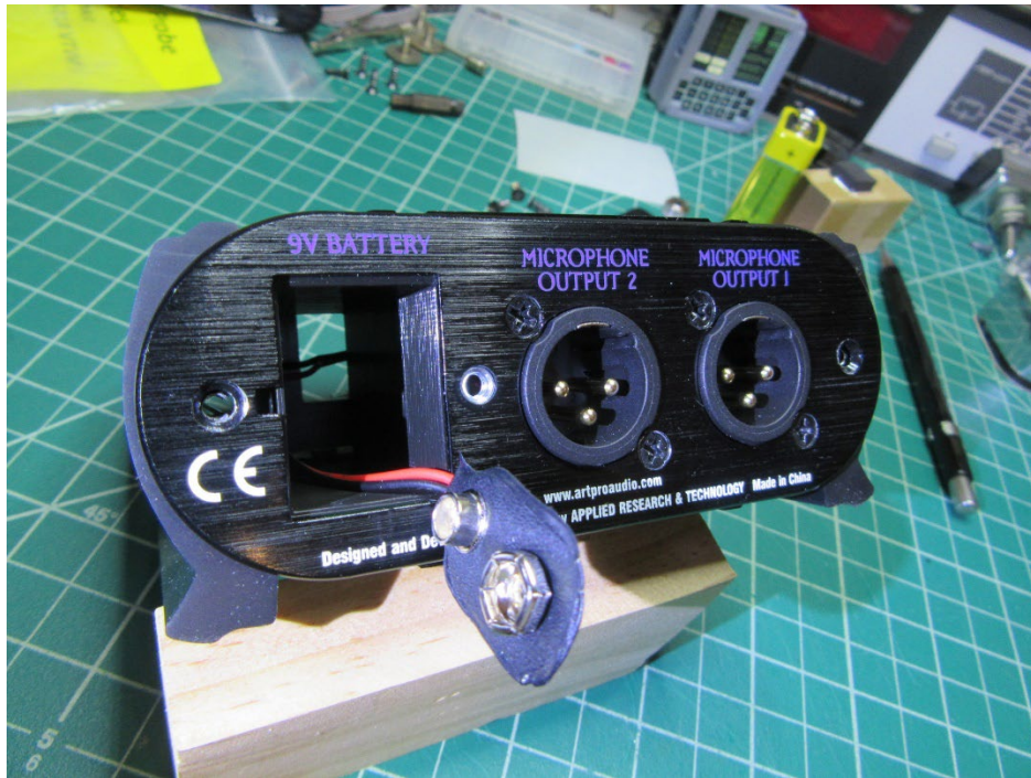
Holder is visible through the rear panel's battery hatch, with the 9V battery connector passing through the holder and out of the hatch
