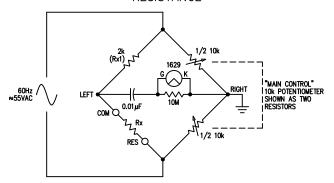
A 60 Hz SINE WAVE, PROVIDED BY THE 55VAC SECONDARY WINDING OF THE TRANSFORMER, ACTS AS THE AC EXCITATION VOLTAGE FOR THE BRIDGE CIRCUIT.
