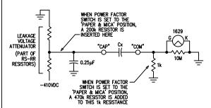
THE CAPACITOR LEAKAGE TEST IS DONE BY APPLYING THE SELECTED TEST VOLTAGE TO A VOLTAGE DIVIDER THAT IS COMPRISED OF THE CAPACITOR UNDER TEST, CX, AND A RESISTOR TO GROUND (IK IN THE DIAGRAM AT LEFT). THE VOLTAGE AT THE CENTER OF THE DIVIDER IS APPLIED ACROSS THE 10M RESISTOR, AND ALSO BETWEEN THE 1629 "MAGIC EYE" TUBE'S GRID AND CATHODE.
