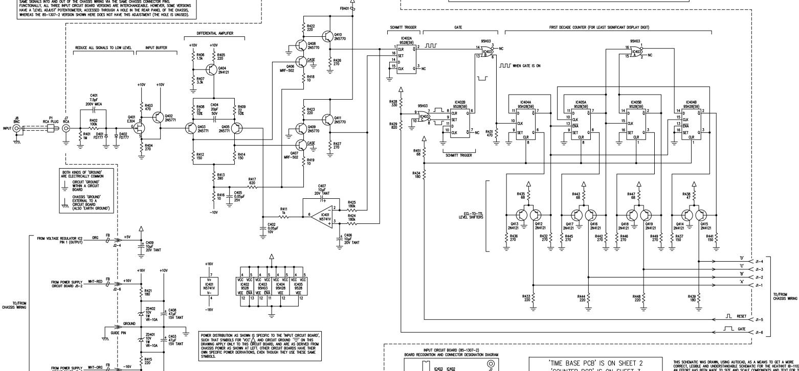
BRIEF CIRCUIT EXPLANATION: THE "INPUT CIRCUIT BOARD" HAS THE TASK OF CONVERTING AN INPUT SIGNAL OF UNKNOWN POLARITY, OFFSET, SQUARE WAVE SIGNAL WITH CLEAN, FAST RISE AND FALL TIMES. R401
