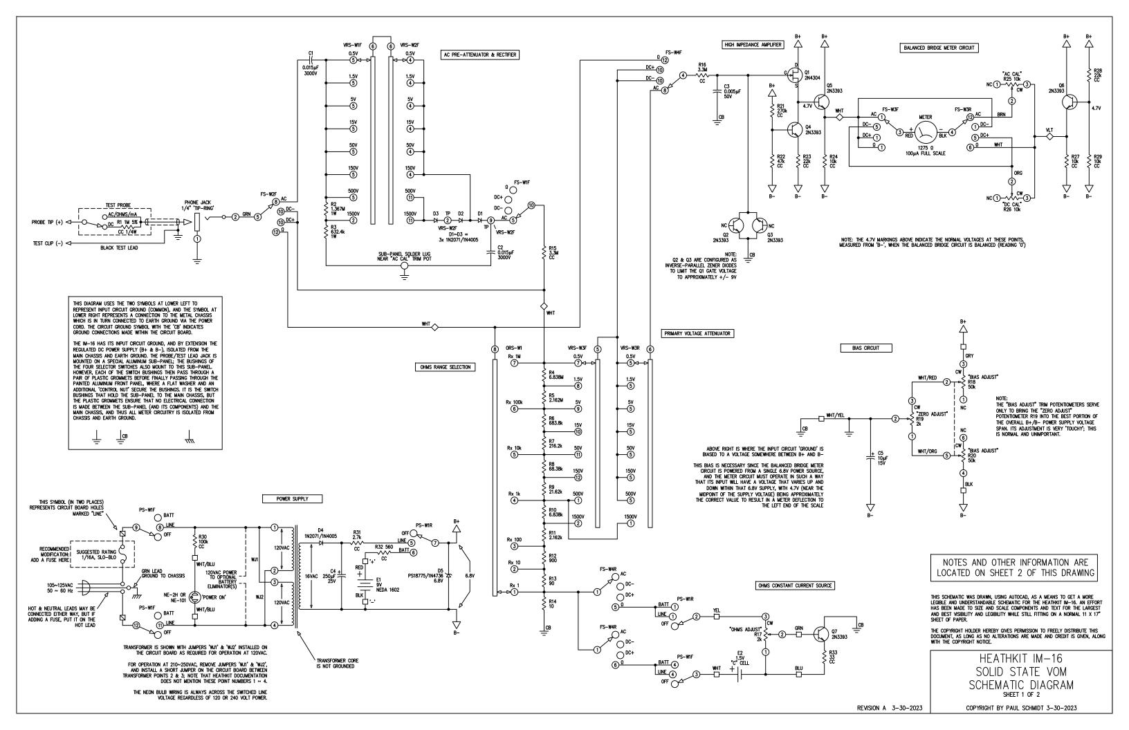
THE VOLTAGE BEING MEASURED IS APPLIED ACROSS A VOLTAGE DIVIDER COMPRISED OF THE 1M OHM RESISTOR 'R1' IN THE PROBE AND RESISTORS IN THE PRIMARY VOLTAGE ATTENUATOR (R4~R14). THE VOLTAGE RANGE SWITCH 'VRS-W3F' TAPS OFF FROM THE APPROPRIATE POINT IN THE VOLTAGE DIVIDER (DEPENDING ON WHICH VOLTAGE RANGE IS SELECTED), AND THIS IS APPLIED TO THE HIGH IMPEDANCE AMPLIFIER (SEE BELOW).
