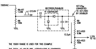
THE TOTAL AC VOLTS PRE-ATTENTUATOR IS COMPRISED OF RESISTORS ADDING UP TO 1.37M. BECAUSE IN THE 1500V RANGE THE ATTENUATOR IS TAPPED AT NEAR ITS BOTTOM. THE ATTENUATION RESULTS IN 151.5VAC AT THIS POINT. AS IN THE EXAMPLE ABOVE, THIS NEEDS TO BE CONSIDERED AS A PEAK VOLTAGE, SO, MULTIPLYING BY 1.41 GIVES 213.6Vp. BECAUSE OF THE ACTION OF THE RECTIFIER/DOUBLER, THE AC IS CONVERTED TO A DC VOLTAGE EQUIVALENT TO THE PEAK-TO-PEAK VALUE Vp X 2. OR 427.2Vpp, GIVING 427.2VDC.
