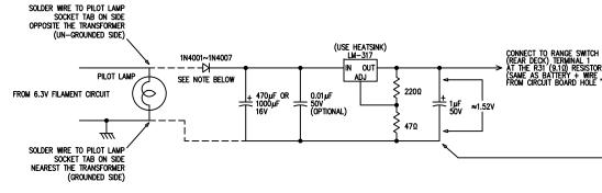
CIRCUIT. AND SHOULD NOT BE MADE AGAIN SEPARATELY FOR THIS BATTERY ELIMINATOR THIS SECTION OF THE DRAWING DESCRIBES HOW TO BUILD AND INSTALL A SIMPLE, RELIABLE
