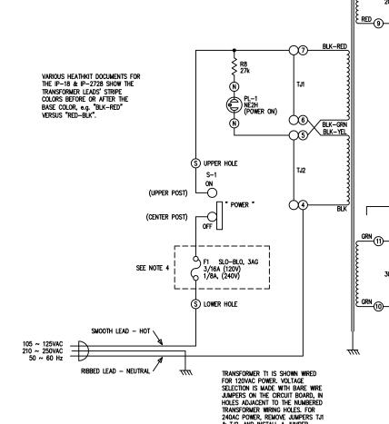
& T.I2 AND INSTALL A JUMPER BETWEEN THE HOLES ADJACENT TO NUMBERED HOLES 5 & 6.
